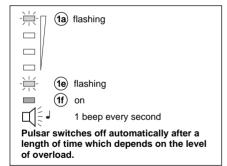
**Note:** overload occurs if the load consumption is greater than the rated power of **Pulsar**.
