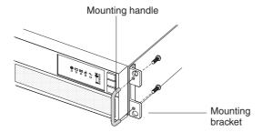
10. Slide the uninterruptible power supply or extended battery module into the rack cabinet. Make sure that you install the extended battery module below the uninterruptible power supply.
