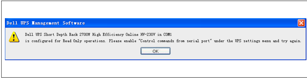
Figure 82. UPS is Set to Read-Only Message
